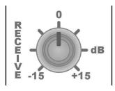
It adjusts in the +/- 15 dB range the level of the signal <u>incoming from telephone caller</u> via the external telephone hybrid.
