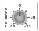
It adjusts in the +/- 15 dB range the level of the signal <u>incoming from telephone caller</u>.
