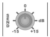
It adjusts in the +/- 15 dB range the level of *mix-minus* signal which is sent to the telephone caller via the external telephone hybrid.
