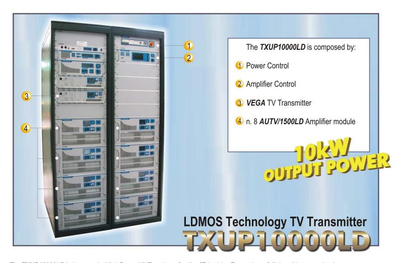
The TXUP10000LD belongs to the High Power UHF products family of Television Transmitters fully in solid state technology.
